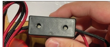
1. Unscrew the two screws holding the black box together
