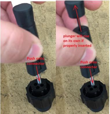
b. **Note**: It will be more difficult to remove female connectors. Is you are having difficulty inserting the extractor, try twisting slightly while inserting.
