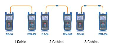
Application note: When performing multimode testing, it's specified to add a mandrel ring to the test cord that's plugged into your light source. This is for launch condition stability and test result accuracy.
