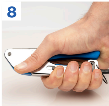
8. With the connector in place, squeeze the handle of the CTF-180M to crimp the COAX connector.
