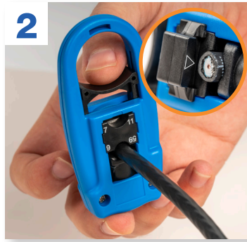
2. Position the blade cartridge so that the 59 and 6 are facing the bottom of the tool (opposite of the ringing handle).
