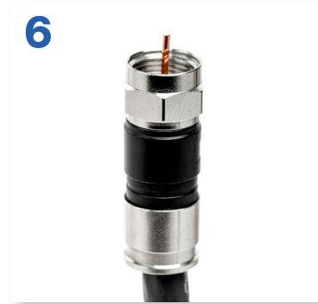
6. Next, push an RG6 connector onto the cable until the dielectric reaches the top of the base of the connector.
