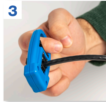
3. Release the lever and rotate the CST-92 around the cable 3 times in each direction.
