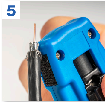
5. Using the hook and loop strip on the side of the CST-92, brush all the exposed braid downward, away from the center conductor.
