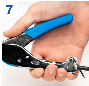
7. Place the connector (with it inserted into the COAX cable) into the compression tool.
