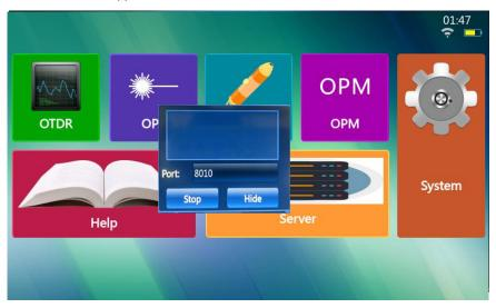
Click any of the six buttons of [OTDR], [Optical power meter], [Optical source], [VFL], [Server] and [Help] in the interface to enter the corresponding module.
