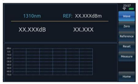
[Wavelength]: Change the test wavelength of the power meter.
