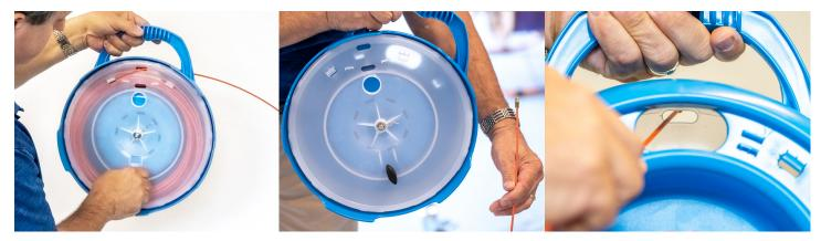
4. Fix this end to the clear plastic backing. 5. Reel the fish tape back in.
