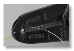
Strips & cuts the most commonly used solid and stranded wires with center conductors from 20 AWG - 30 AWG (0.81 mm - 0.25 mm). This wire stripper features the following:
