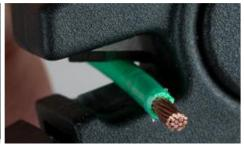
With their innovative squeeze and strip design, these self-adjusting wire strippers automatically grasp and strip insulation off wires. These tools are perfect for stripping thick or thin wall insulations such as PVC or other wires at specific strip lengths without having to make tedious adjustments. These self-adjusting wire strippers features the following:
