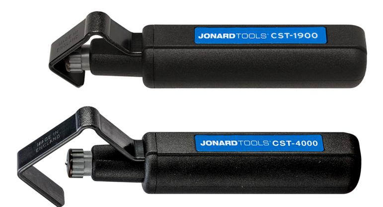
The **PATENTED** CST-1900 and CST-4000 Round Cable Strip & Ring Tools are designed for fast and precise removal of cable jackets from round cables. The CST-1900 removes cable jackets 3/16" to 1 1/8" (4.5 mm to 29 mm) in diameter and the CST-4000 removes cable jackets 3/4" to 1 5/8" (19 mm to 40 mm) in diameter. These round cable strippers feature the following:
