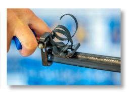
Designed to shave thick jacketed cable, such as Corning's armored and non-armored RocketRibbon® cable, this tool is perfect for making access windows on cables 0.47" to 0.87" (12 - 22 mm) in diameter. This tool also features the following:
