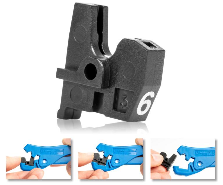
This is the replacement blade cartridge for the BTR-6 Buffer Tube Ringing Tool. This replacement blade cartridge is used for buffer tubes between 1.2 - 6.0 mm in diameter. The blade is a factory-fixed hardened steel blade for precise nick-free jacket entry.
