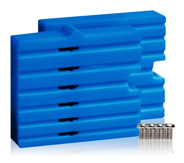
This is the replacement blade set Mid Span Slitter for Hexatronic Stingray Fiber Cables and comes with (2) blade cartridges. This replacement blade set is for cable diameters from 1.1 mm to 1.6 mm. The blades are made for long term use and last for up to 5,000 slits/cuts.
