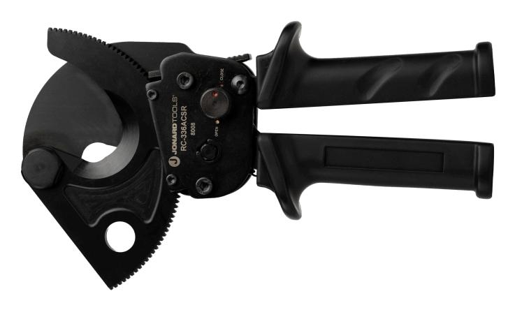
Designed for heavy-duty use, This cable cutter is designed to cut 336 MCM (170 mm²) ACSR, 400 MCM (202 mm²) copper, or 600 MCM (304 mm²) aluminum cables, and most cables up to 30mm in diameter. This cable cutter features the following:
