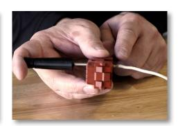
Compatible with nearly all AMP-style pin connectors between contact sizes 16-20, this tool is perfect for extracting AMP CPC pins from the back of connector blocks. This insertion tool features the following:
