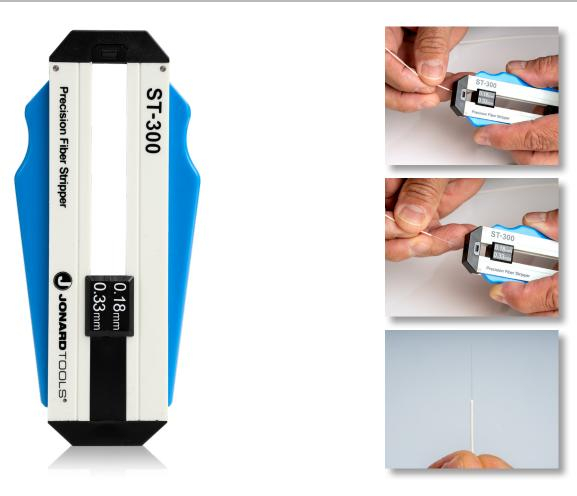
Designed for precision fiber optic stripping, this tool is perfect for stripping the 180 - 330 micron acrylate coating to expose the 125 micron glass fiber of fiber optic cables. This precision fiber stripper also features the following:
