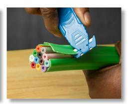
Designed with slim safety heads and high carbon steel blades, this microduct sheath slitting tool is perfect for slitting the sheaths off microduct bundles to access the microducts inside. This sheath slitting tool also features the following:
