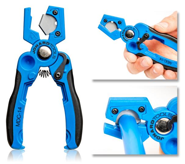
Designed to cut microducts cleanly and straight, this microduct cutter is perfect for cutting most microducts including tubing made from PVC, Nylon, and other materials up to 14 mm (9/16") in diameter. This microduct cutter features the following:
