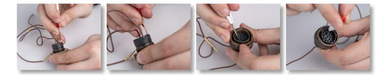
This tool is perfect for inserting and extracting size 20 front release contacts made by most manufacturers. This insertion tool features the following:
