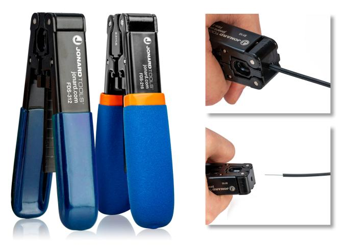
Specifically designed to strip FTTH drop cables sized 1.6 mm (**FDS-216**) and 3.1 mm (**FDS-312**) by 2.1 mm. These drop cable strippers strip the outer jacket of drop cables and cuts the strength members to expose the fiber inside. These drop cable strippers feature the following:
