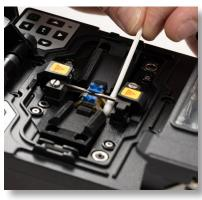
Made with lint-free cotton, these cotton swabs are perfect for cleaning dirt, dust, and debris from the V-groove of your fusion splicer. These cotton swabs also feature the following:
