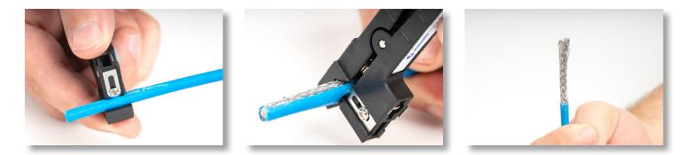
Designed to slit COAX, network, and other types of cables 3/16" - 5/16" (4.8 - 8.0 mm) in diameter, this cable slit and ring tool is perfect for any CATV technician. This cable slit and ring tool features the following:
