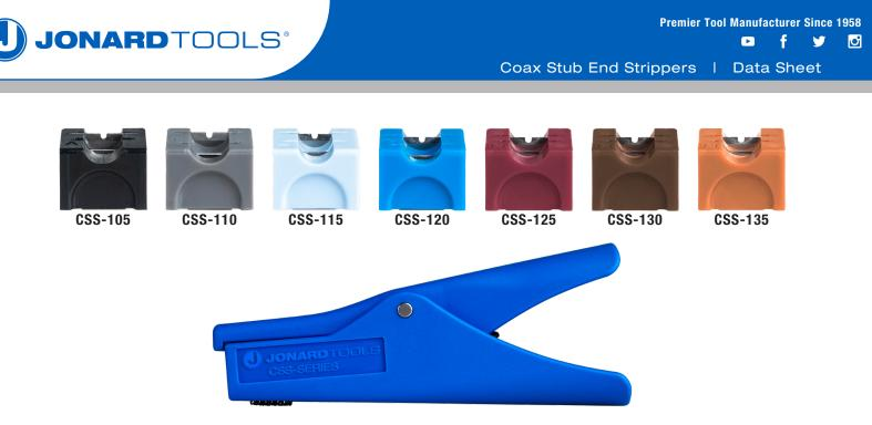
The CSS Series tools are coaxial cable strippers specifically designed to strip a stub end of a coax cable in a wall outlet box, which eliminates the need to run new cable, saving time and money. Each strips RG-59 and RG-6 cables to specific braid and center conductor lengths shown in chart below. The built-in strip stop insures the strip lengths are consistent. VELCRO® strip on bottom of tool is used to fold back braid on cable after being stripped.
