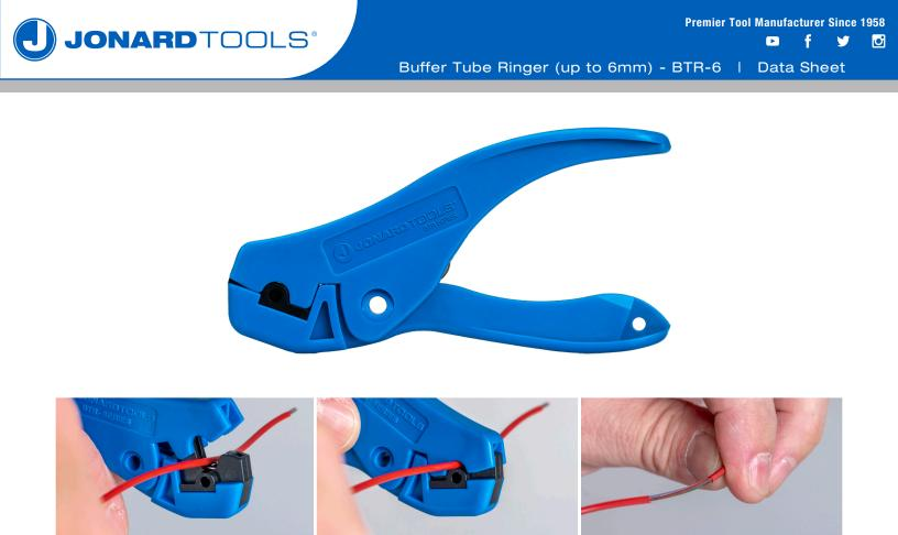
The Jonard Tools **BTR-6** Buffer Tube Ring tool provides quick access to fibers inside buffer tubes from 1.2 mm to 6 mm in diameter and will work with buffer tubes with wall thicknesses from 0.2 mm to 0.5 mm. The tool is light and durable with a hardened steel blade for long life and includes a hole for tethering.
