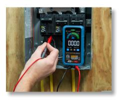
Intelligent, auto-function volt meter is capable of gauging both the required range and the required function based on the test lead input, providing the simplest experience and the most accurate results. Simply plug in the leads and connect to your test subject and let the AMM-600 take the guess work out of testing.
