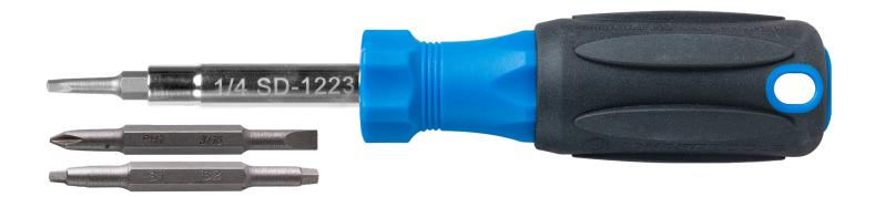
The Jonard Tools 6-in-1 Multi-Bit Robertson Screwdriver eliminates the need for multiple tools in your belt. This tool can be configured to 6 types of driving heads: #2 Phillips Head & 9/32" Cabinet Slotted Head, S1 & S2 Robertson Head, 5/16" & 1/4" Nut Driver Head. This screwdriver features the following:
