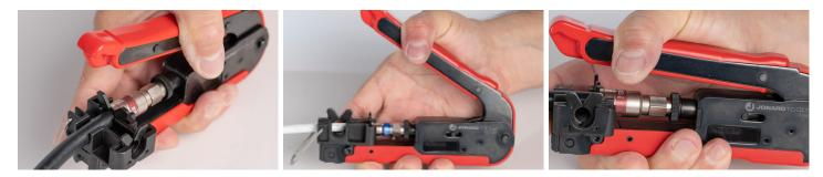
Using specially designed jaws to hold connectors in place while compressing, this **PATENTED** CTF-360 is designed to hold and compress connectors requiring a full 360 degree support. Perfect tool for short F connectors for RG59/6 cables and F connectors for RG7/11 cables. This tool also features the following:
