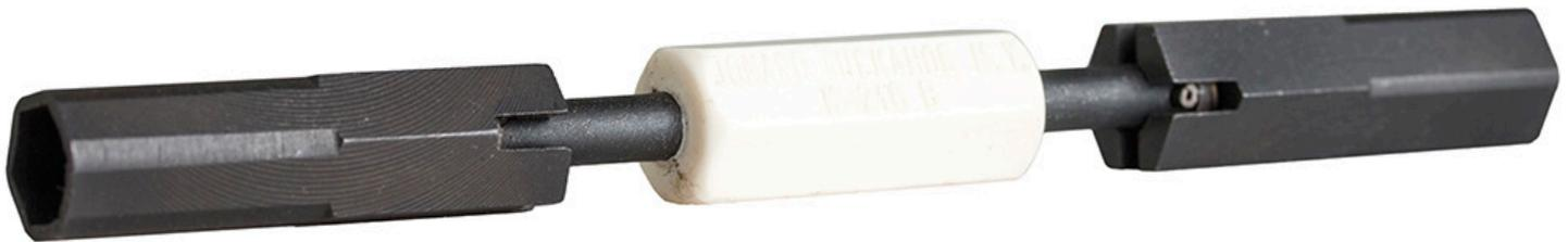
Standard can wrench with 3/8" & 7/16" sockets plus a built in .031" screwdriver in each end. The tool is spring loaded for simultaneous nut and screw adjustments. Extended it measures 6-1/2" long and retracted just 5-3/8" long.
