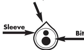
4. Tighten the collet by rotating the collet nut in the counterclockwise direction. The tool is now ready for use. To make a wire wrapped connection, follow the instructions and helpful hints on the pages ahead.
