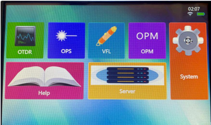
Click any of the six buttons of [OTDR], [OPM], [OLS], [VFL], [Server] and [Help] in the interface to enter the corresponding module.
