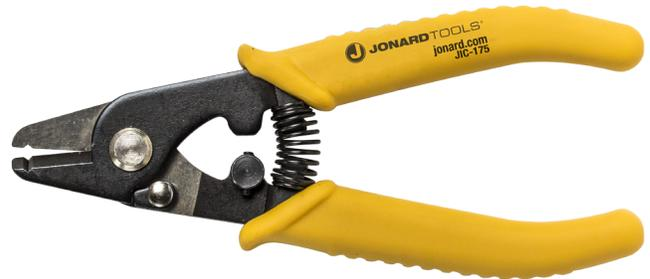
**JIC-125 Fiber Optic Stripper and JIC-175 Fiber Optic Stripper:** Used for stripping the 250 micron coating from the cable down to the glassfiber without any nicks or scratches
