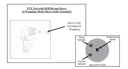
To change to unwrapping mode, ensure that the wrap/unwrap switch on the PTX tool is set in the UNWRAP position. Then, follow instructions in figure 1.
