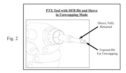
To change back to the wrap mode, first ensure that the wrap/unwrap switch on the power tool is set in the WRAP position. NEXT, ENGAGE THE TRIGGER ONCE TO RE-INDEX THE BIT TO THE PROPER POSITION. Then, pull the sleeve out approximately 1/4" and rotate the sleeve in either direction 180°, then release. The spout on the sleeve should be in the 12:00 position and the sleeve should be locked in place.
