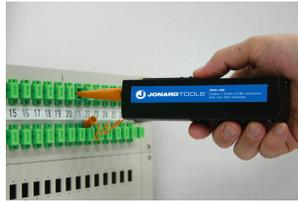
To clean end faces of connectors, open the top of the cap exposing the connector adapter. Insert connector into adapter and pull connector towards the tool until you hear an audible click. The cleaning process is now complete.
