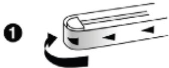
2. Dual Rotational tip provides quick, repeatable and superior ferrule end face cleaning
